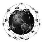
GPS uses a constellation of satellites that continually send radio signals to the earth. Your present position is determined by receiving signals from up to 16 satellites and measuring the distance from the satellites.
